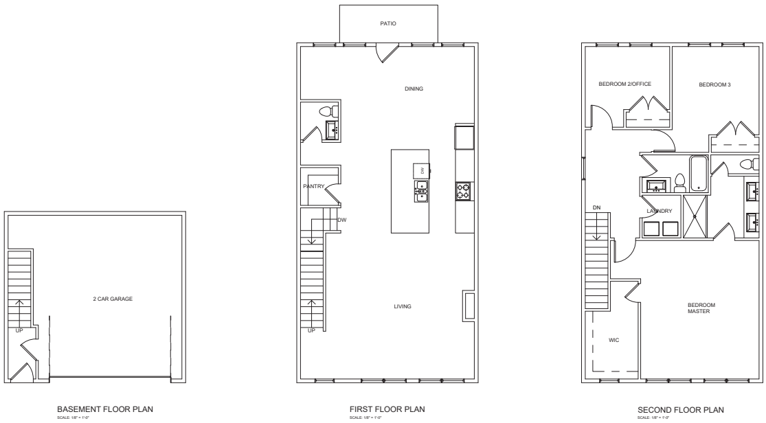
TYPE A - 24 X 45-TWO CAR GARAGE-3 LEVEL BASEMENT-3 BEDS - 2,233sf REAR ENTRY BASEMENT UNITS
