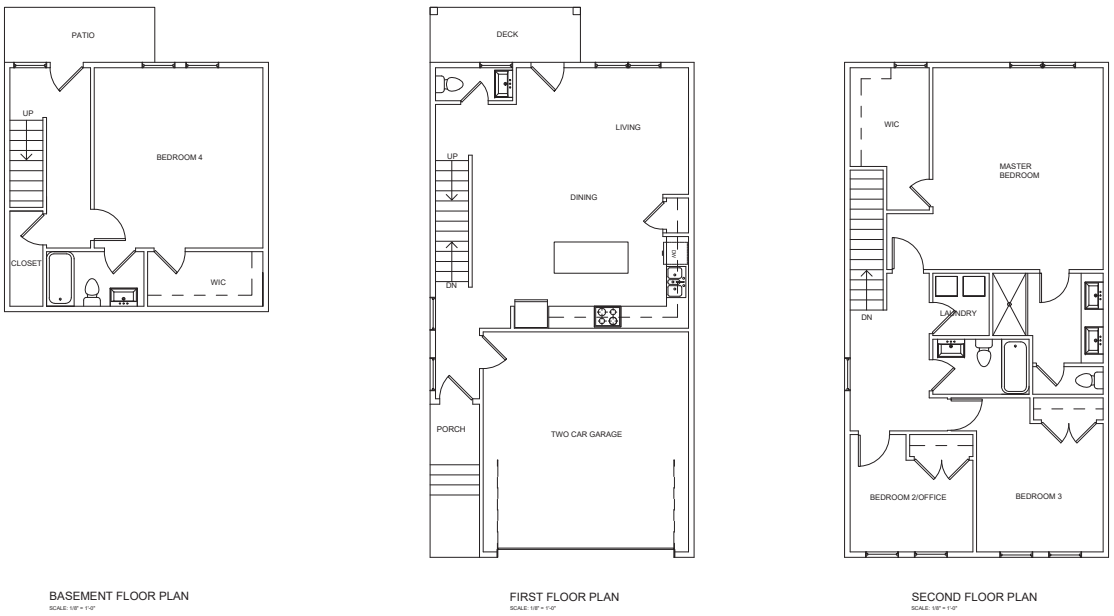
TYPE B - 24 X 45-TWO CAR GARAGE-3 LEVEL BASEMENT-4 BEDS - 2,243sf FRONT ENTRY GARAGE UNITS
