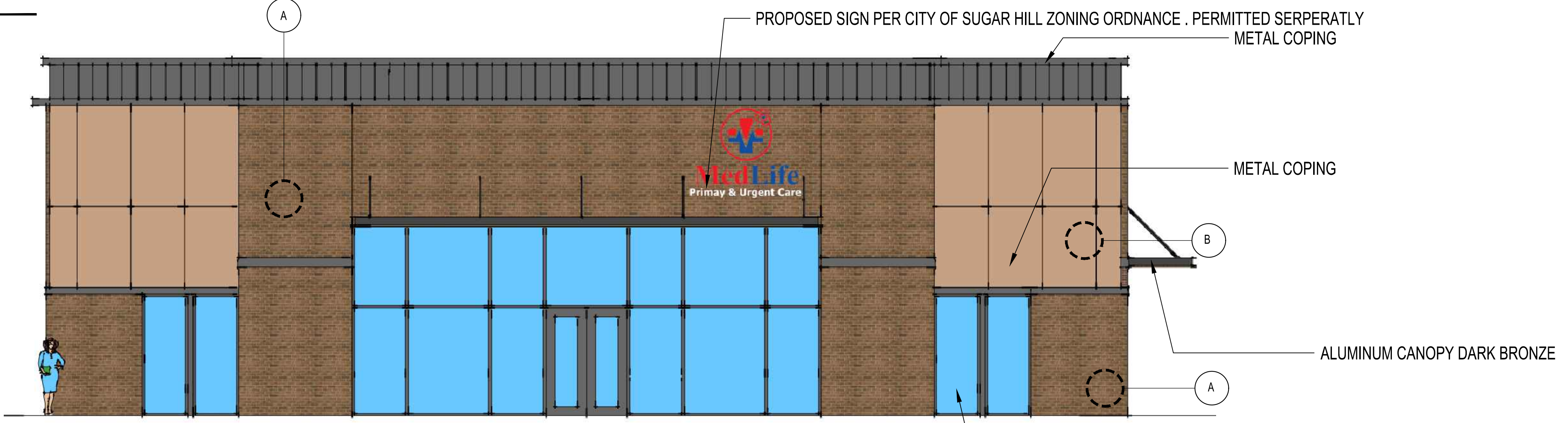
4 NELSON BROGON BLVD EXTERIOR ELEVATION 3/16"=1'-0"
